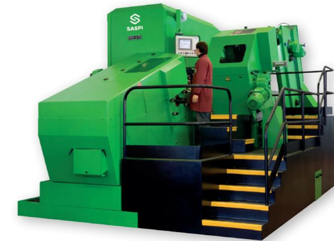
This machine combines a thread-rolling machine and a Saspi pointing machine in order to carry out the following tasks in a single feed processes of chamfering and threading or drilling and threading of parts.
