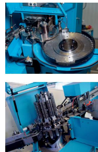
This machine incorporates a system for inserting washers into the parts before rolling.
