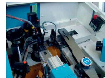
These are secondary operation machines for the fastener industry in which their main function is the facing and chamfering of parts, their flexibility allows numerous operations.
